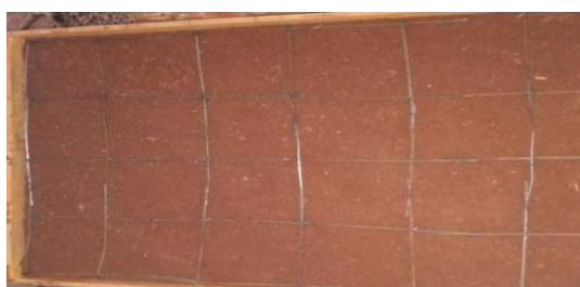
Fig :4 compacted natural soil + reinforcement with 15cm spacing
