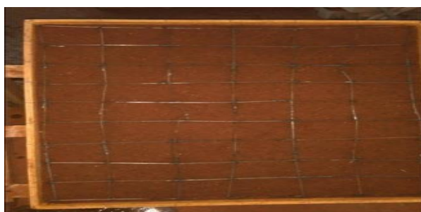
Fig : 5 compacted natural soil + reinforcement with 10cm spacing
